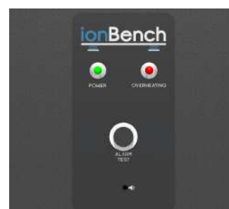
Overheating temperature alarm
