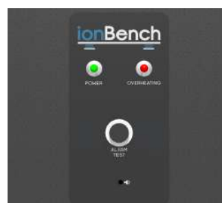
Overheating temperature alarm
